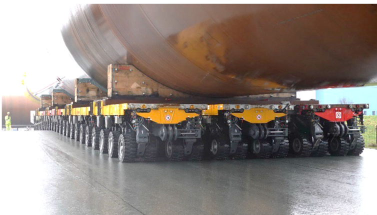
Figure 6: Transport of a monopile by SPMT over a dike crossing
